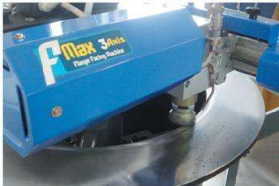
Surface facing finish on a flange coupling.
