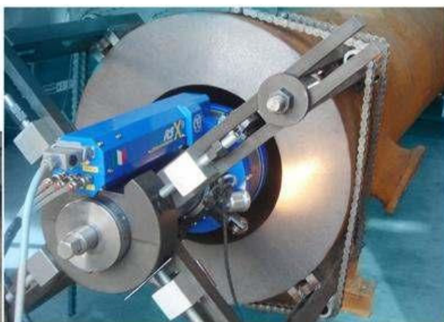
Machining on ingot mould of length 5600 mm diameter 600 mm
