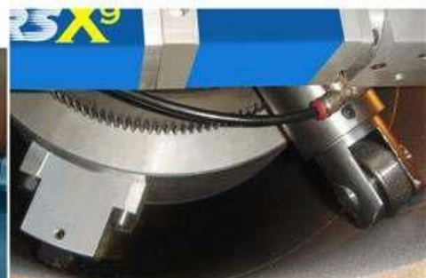
Self-centring support with pneumatic expansion
