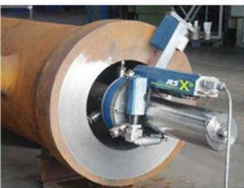
Kit for facing with a motorized feed
