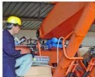
Reconditioning and realignment of the chassis holes without disassembling the arm. It's evident from the pictures that the use of our machines simplifies the most difficult operations.
