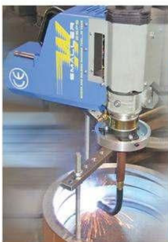
Overlay welding on Ø 380 mm
