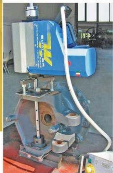
Reconditioning of the steering axle housing
