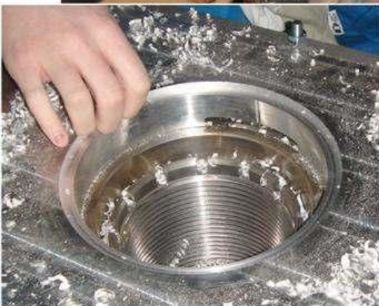
Threading diameter 230 pitch 6
